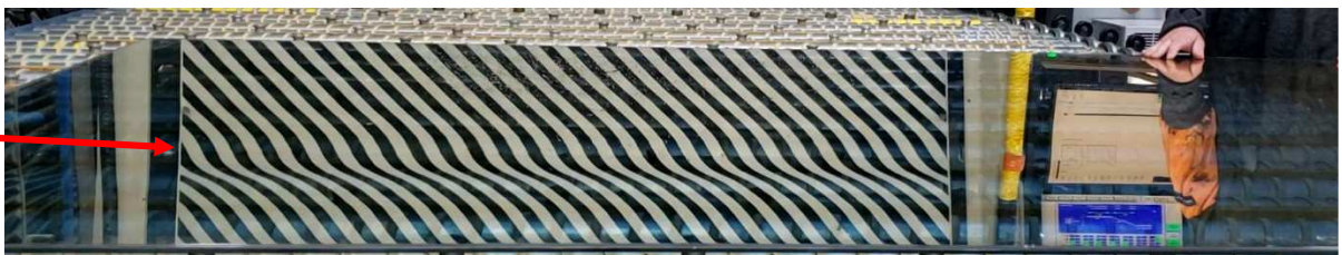
Photo #24: Localized vertical distortion was confirmed in project glass sample D07 after rotating it counterclockwise 90°.
