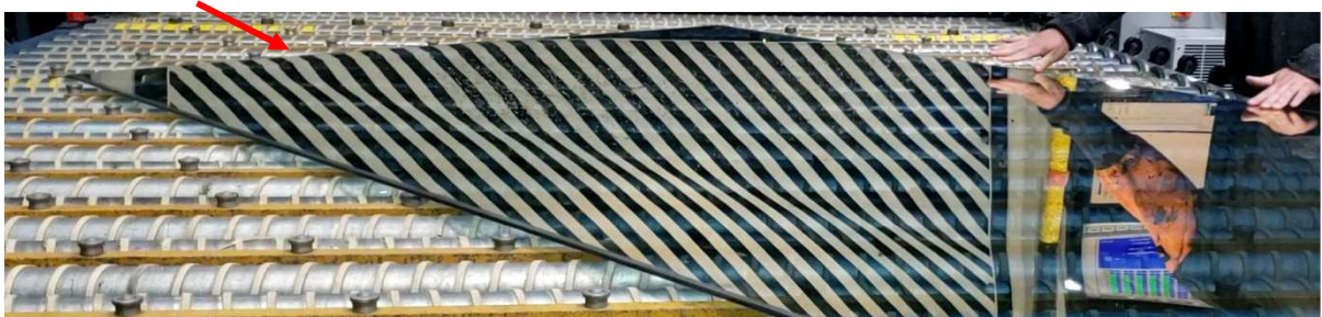
Photo #22: Localized vertical distortion starts to appear in project glass sample D07 after further rotation of the glass.
