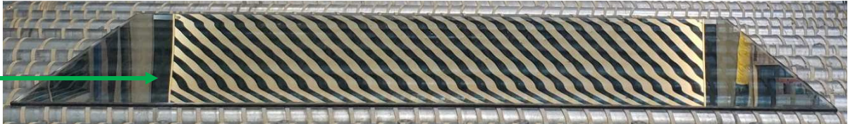
Photo #16: Zebra board visual evaluation of project glass sample B13 in Group 3. Edge kink was observed, which is to be expected in heat-treated glass.
