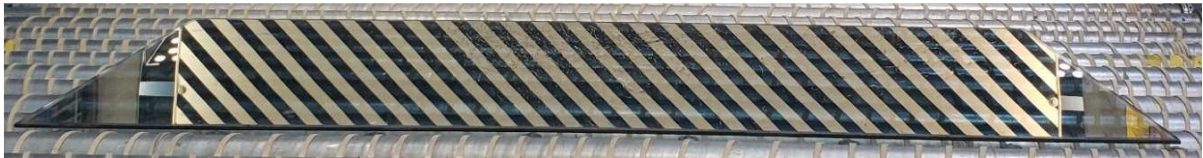
Photo #17: Zebra board visual evaluation of project glass sample B17 in Group 3. Edge kink was not observed, which is unusual for heat-treated glass.
