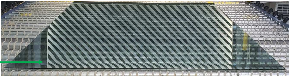
Photo #18: Zebra board visual evaluation of the baseline control glass sample for group 4. Edge kink was observed, which is to be expected in heat-treated glass.
