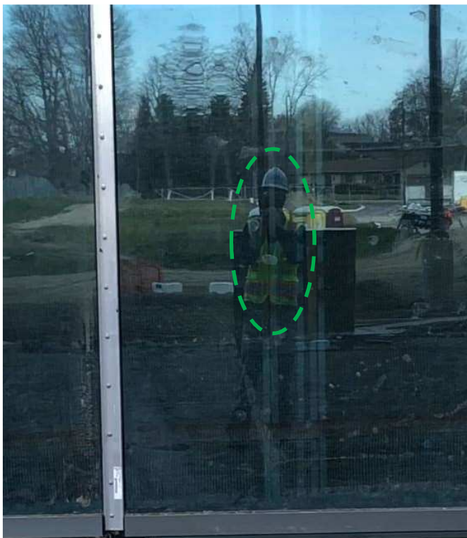
Photo #6: Non-distorted reflected image of a person after moving slightly further towards the right.
