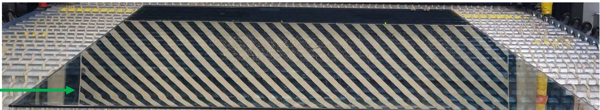
Photo #19: Zebra board visual comparison evaluation of project glass sample D07 in Group 4. Edge kink was observed, which is to be expected in heat-treated glass.
