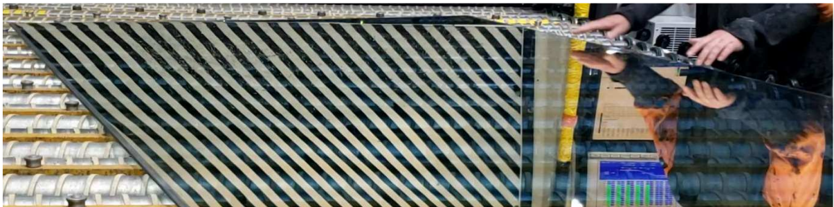
Photo #21: Vertical distortion not observed in project glass sample D07 when glass was slightly rotated counterclockwise.
