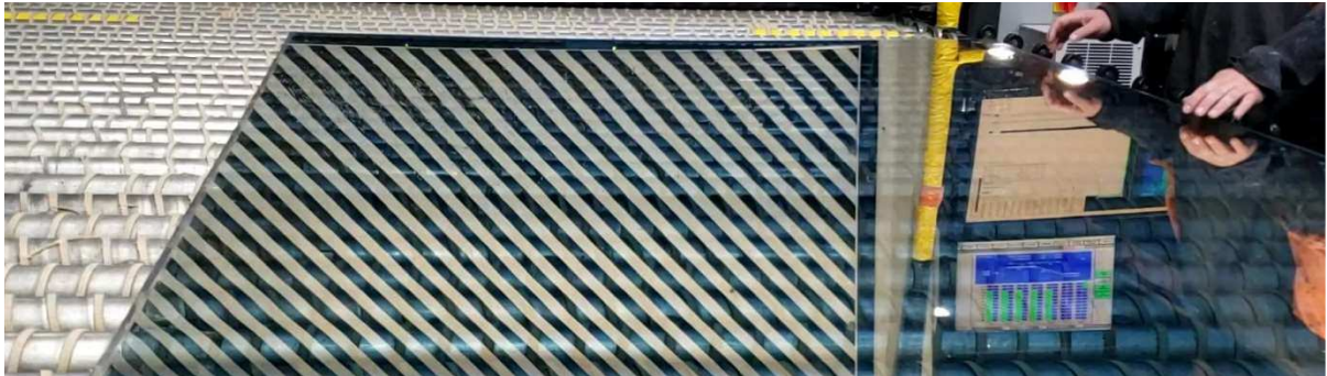
Photo #20: Vertical distortion not observed in project glass sample D07 as viewed in direction of travel through oven.
