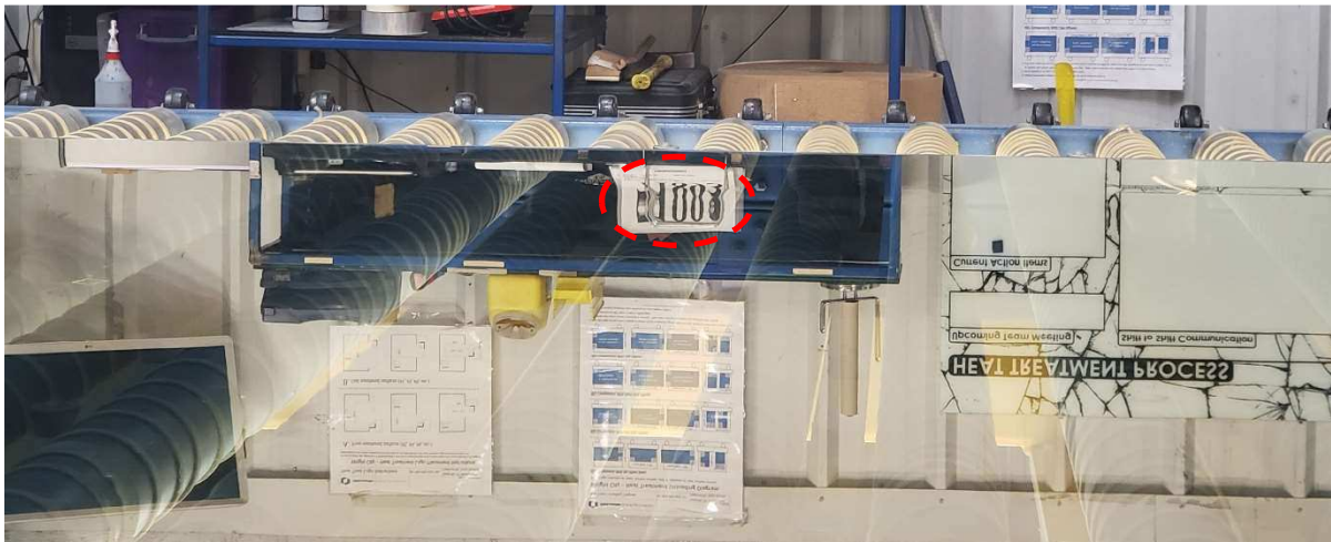
Photo #37: Side view of a distorted reflected image (at the localized vertical distortion) on project glass sample A19.
