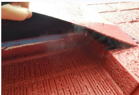
PHOTOGRAPH 6. Poorly bonded transition membrane, with tracer gas leak during diagnostic airtightness testing.
