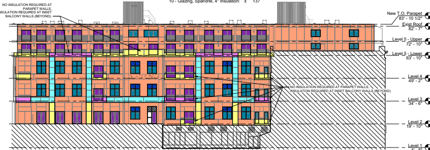
3 WEST ELEVATION - COURTYARD SCALE: 1/16" = 1'-0"
