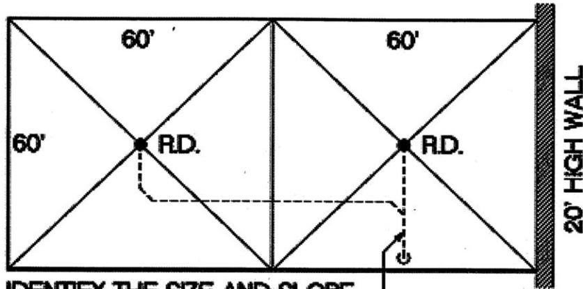
IDENTIFY THE SIZE AND SLOPE OF THIS SECTION OF ROOF LEADER PIPING
